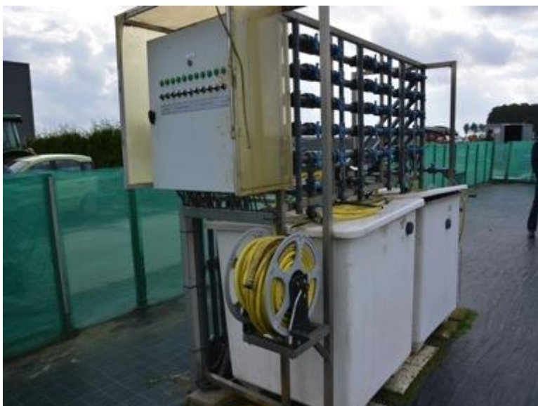
Figure 28. Irrigation control rig for solution hydroponics
